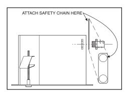
a. Attach the conduit fitting, lock nut, and safety chain bracket.
